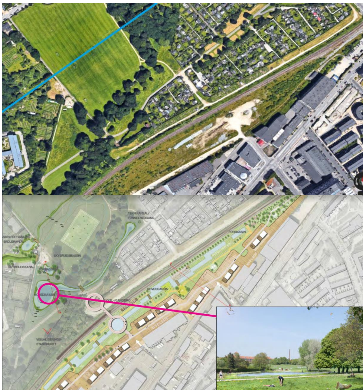
Figure 7: Lersøparken in its current state, with the piped Lygte Å in blue (top image). Bottom image: the proposals for its development as part of Copenhagen's cloudburst plan (Københavns Kommune).
